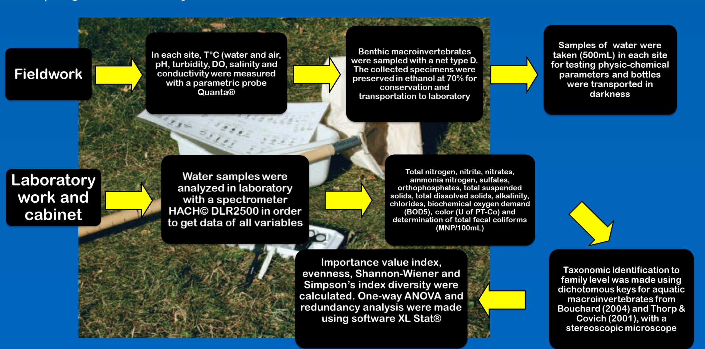
Fig. 2. Process of sampling and analysis of fieldwork, laboratory and cabinet work.
